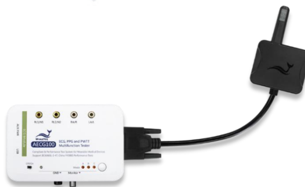
Figure 6: Direct Connection between AECG100 and PPG-2TF-660 2.0
