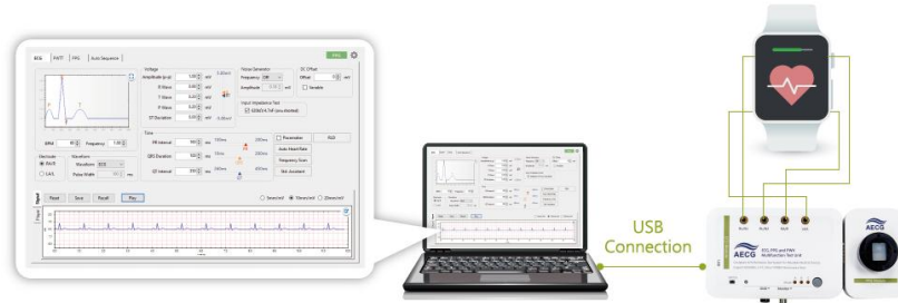
Figure 7: ECG Test Mode Product Wiring Diagram
