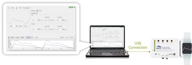
Figure 11: SpO 2 Test Mode Product Wiring Diagram
