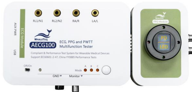
Figure 4: Direct Connection between AECG100 and PPG Module
